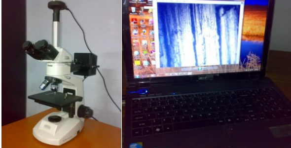
Fig 4. KRUSS Metallurgical microscope used for measuring tool wears
